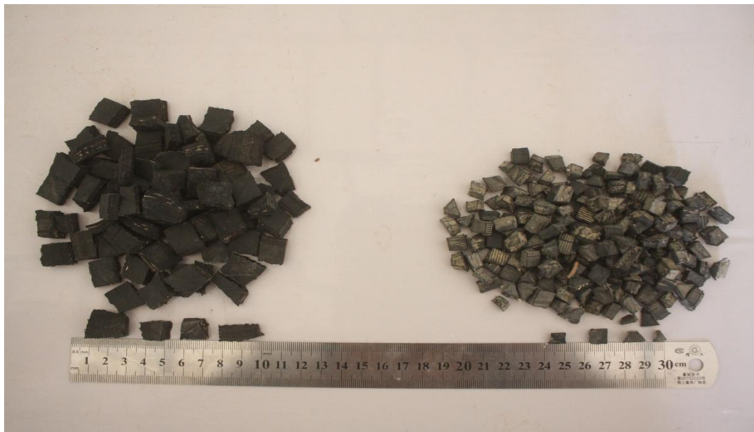
Figure (2): Tire chip size (5-9)mm and size(10-20)mm
