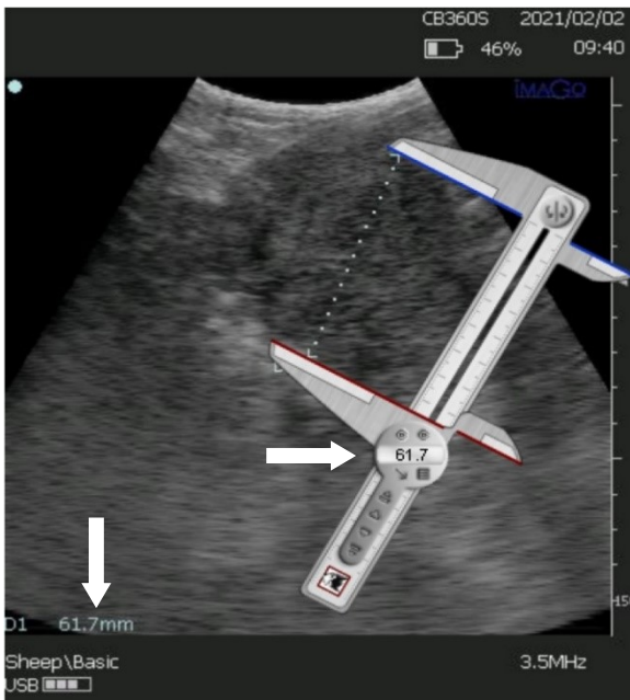
Figure 1: Calibration of the Screen Caliper software through an image of the ultrasonic device with known distances in millimeter.
