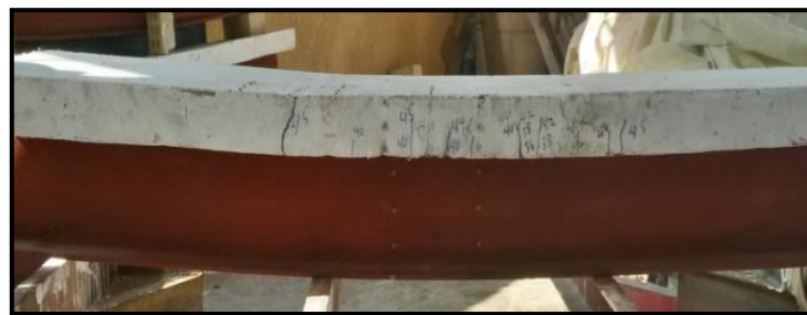
Plate (3) Cracks Pattern for Test Specimens (Continued)
