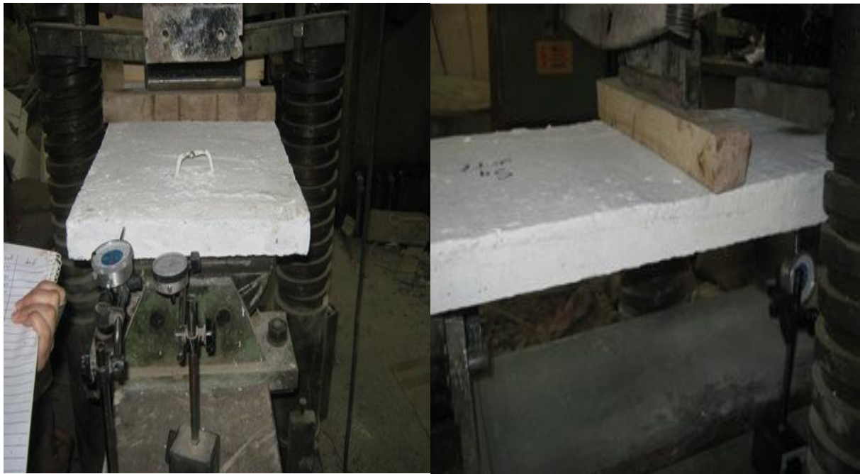
Fig. (4): Arrangement before testing panels.
