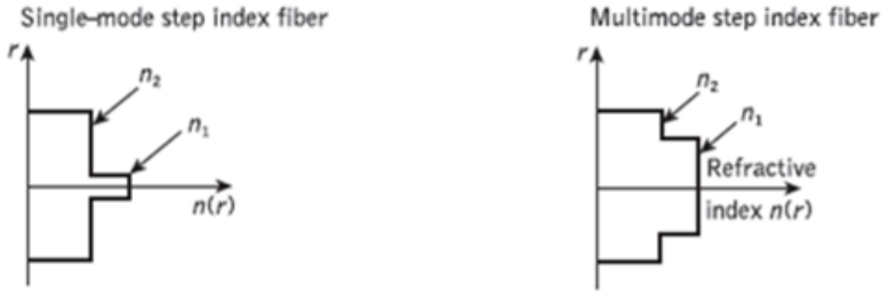
Figure 1. Schematic diagram showing a SM SIF and MM SIF, where r is the radial position [5].
