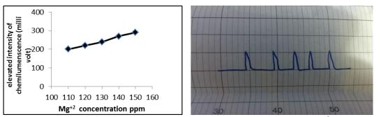
Figure (1) relationship between the intensity of chemiluminescence emission and Mg<sup>+2</sup> concentration
