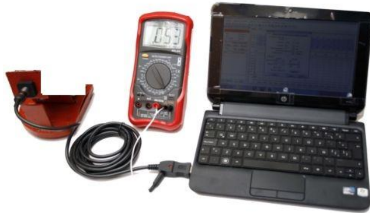
Fig. (2) The USB vibration analyzer used
