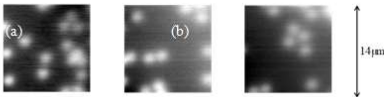
Fig .3. Scanning Hall Probe images of \text{Sr}_2\text{RuO}_4 at three different locations. The sample was cooled in the earth's field. [ T=300\text{mk} , H_{\text{APP}}=0 ]
