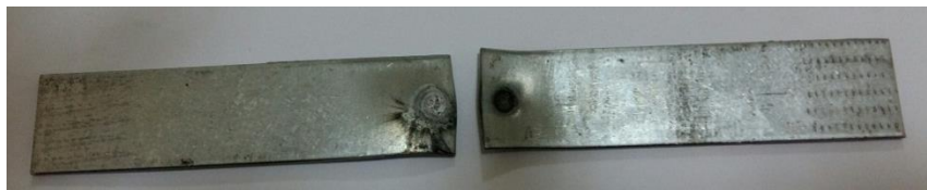
Figure (6): Fractured shear test specimen
