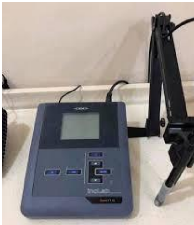
Figure2. Device of conductivity meter
