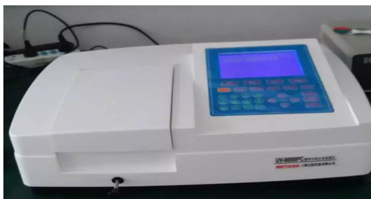
Figure3. Device of UV-Visible Spectroscopy.
