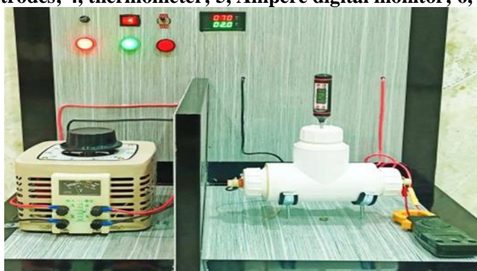
Figure (2): Batch type ohmic heating device
