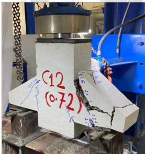
Figure :(15-a) : Mode failure of specimen C_{12}
