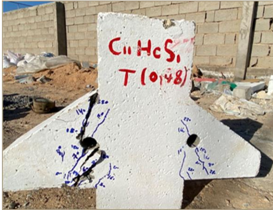
Figure :(14-a): Mode failure of specimen C_{11}
