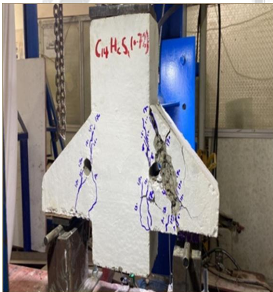
Figure : (17-a) Mode failure of Specimen C 14
