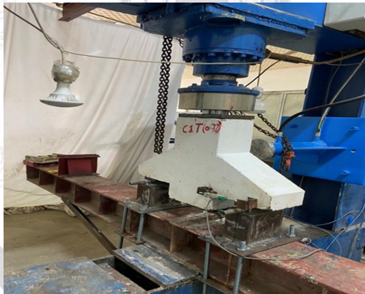
Figure:8 – Test setup with corbel specimen
