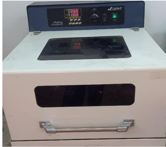
Fig. 2 The Batch-Type Adsorption Unit LabTech Incubator Shaker.
