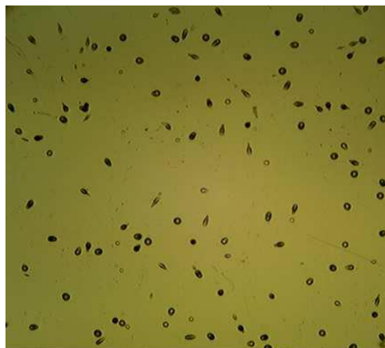
Fig.3: Alpha track registered by CR-39NTDs
