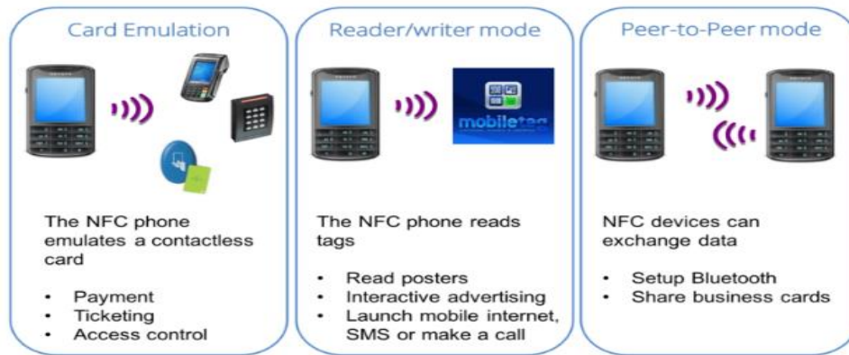
Figure 2 NFC operating mode(source (RFID 4u))
