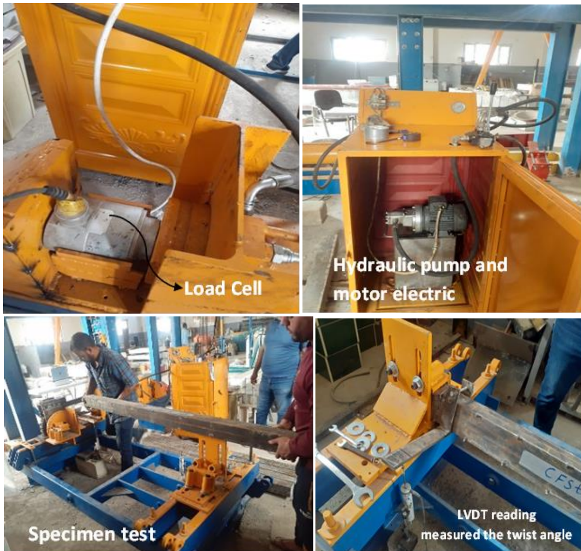
Fig. 11 Steel Tubular Specimens Filled-Concrete Test.
