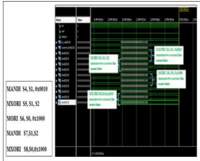
FIG.14. TEST CODE AND WAVEFORM RESULTS FOR LOGIC SIMD INSTRUCTIONS
