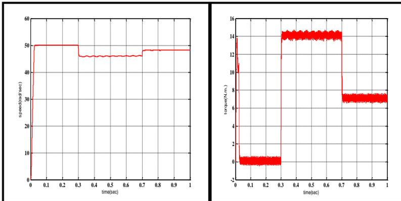
**Figure (11) Speed and torque responses at  $\omega=50$  rad/sec,
