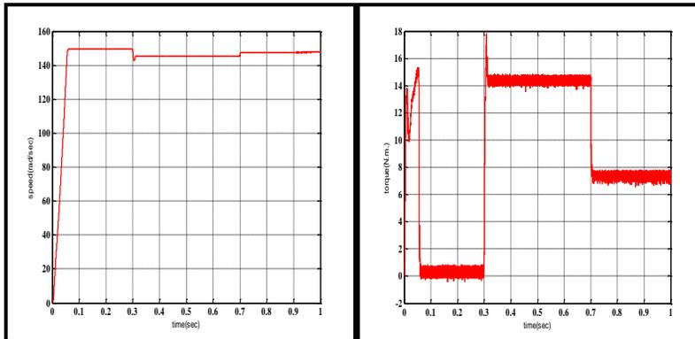
**Figure (9) Speed and torque responses at  $\omega=149$  rad/sec,**
