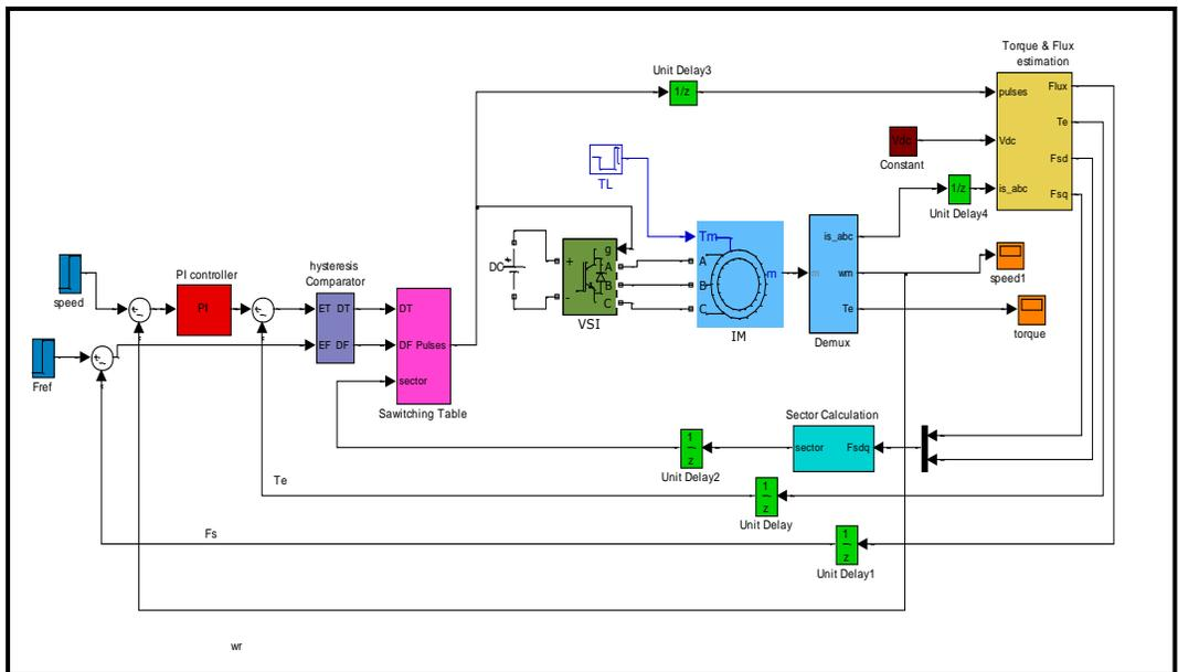
**Figure (8) Simulink program of DTC with conventional PI controller**
