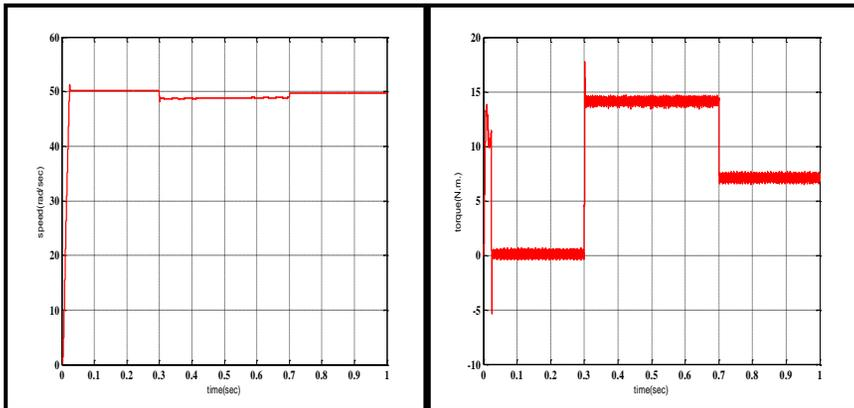
**Figure (14) Speed and torque responses at  $\omega=50\text{rad/sec}$ ,
