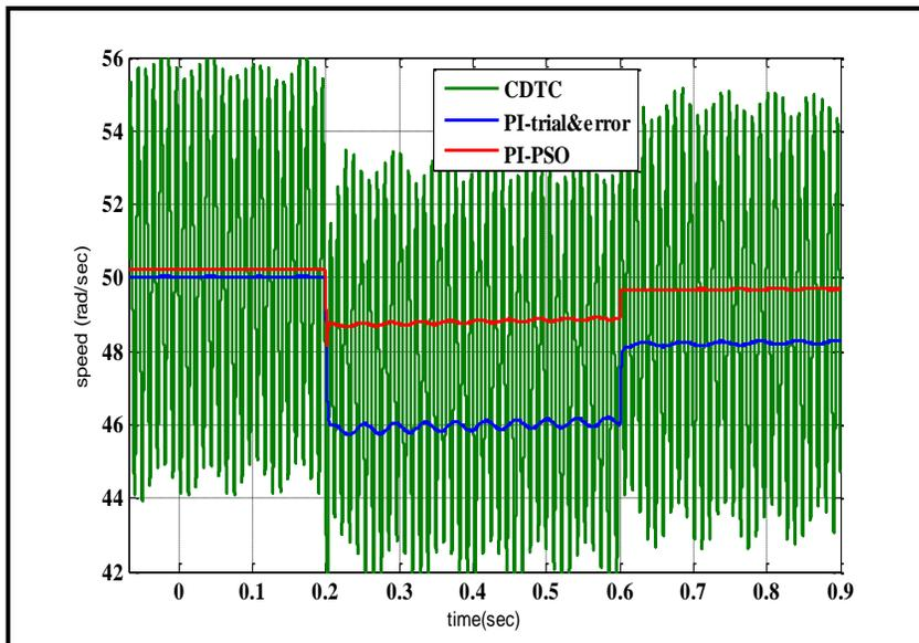
**Figure (17) Speed response at  $\omega=50$ rad/sec.**
