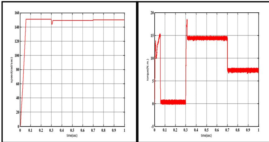
**Figure (12) Speed and torque responses at  $\omega=149$  rad/sec,
