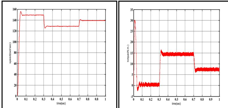
**Figure (5) Speed and torque responses**
