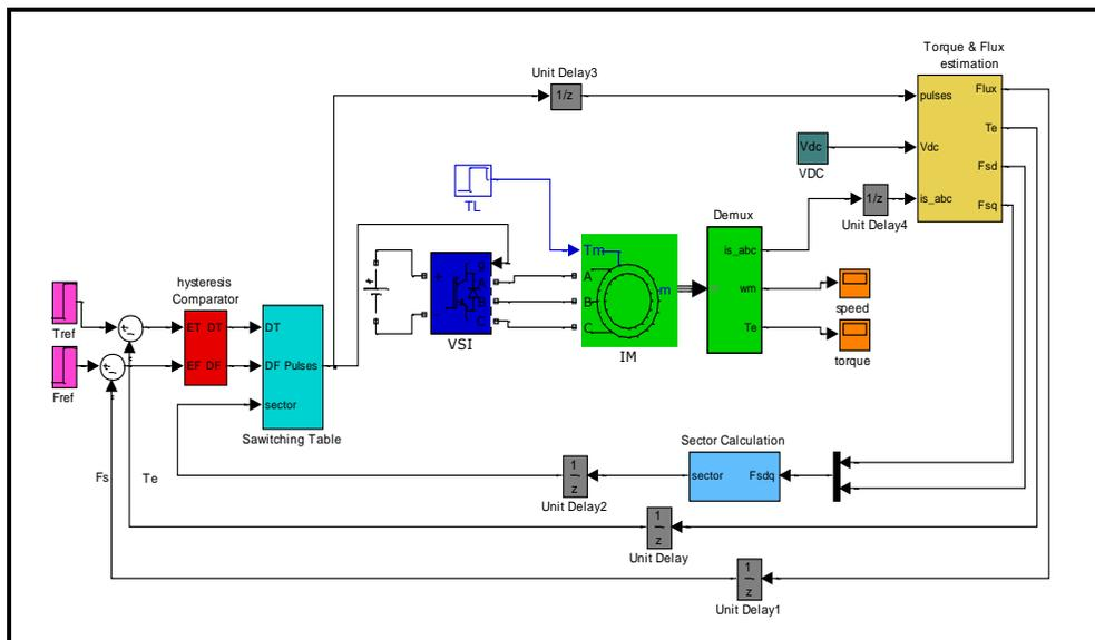
**Figure (4) Conventional DTC circuit**
