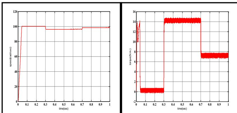
**Figure(10) Speed and torque responses at  $\omega=100$  rad/sec,**
