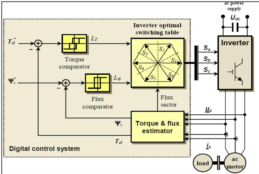
Figure (2) DTC block diagram.
