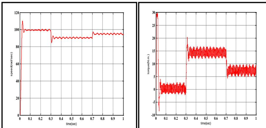
**Figure (6) Speed and torque responses**
