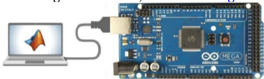
Fig. 10 Interfacing MATLAB on a laptop with Arduino Mega using USB.
