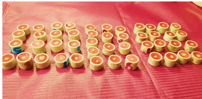
Figure (1): The crowns were mounted in cylindrical plastic tubes (16mm diameter ×14mm depth) with cold cure acrylic resin with the outer buccal enamel surface exposed
