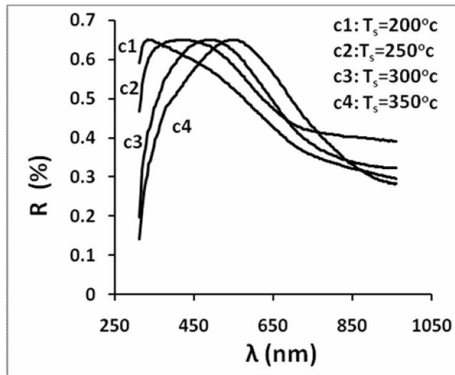
Fig.(5):Spectral behavior of Reflectance for SnS thin films prepared at different Sub. Temp.
