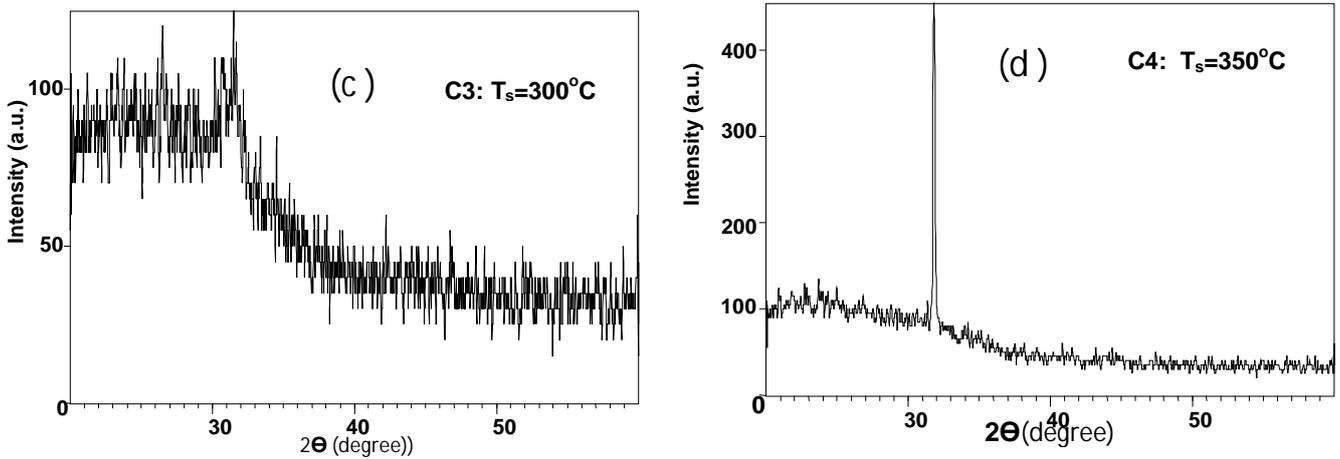
Fig.(1):XRD pattern of SnS thin films prepared at different Sub. Temp .
