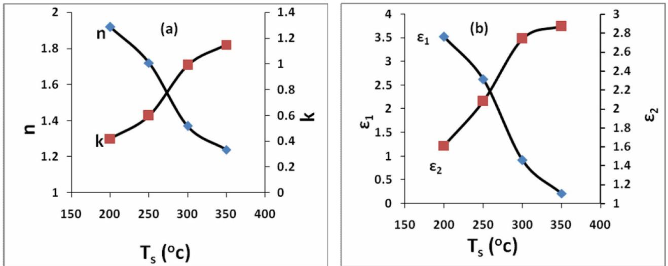
Fig.(9): Optical parameter(a): n, k (b):  $\epsilon_1, \epsilon_2$  as a function of Sub. Temp .
