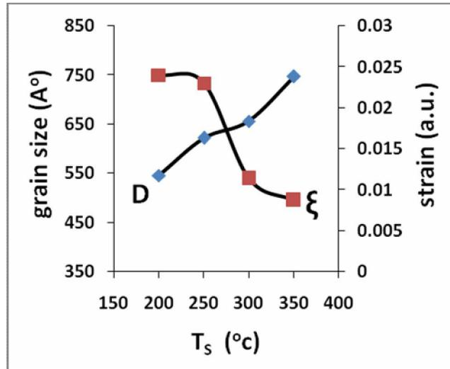
Fig.(2):Grain size and Strain of SnS thin films as function of Sub. Temp.
