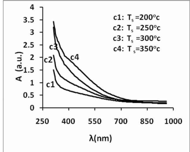
Fig.(4):Spectral behavior of Absorbance for SnS thin films prepared at different Sub. Temp.
