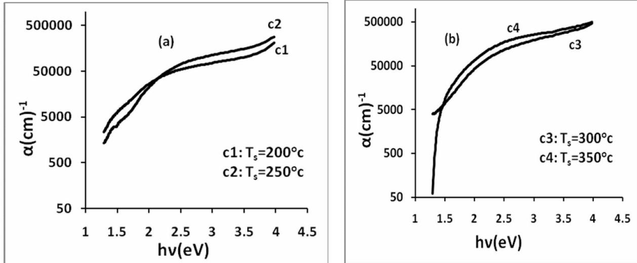
Fig.(6):Absorption Coefficient ( $\alpha$ ) for SnS thin films prepared at different Sub. Temp.
