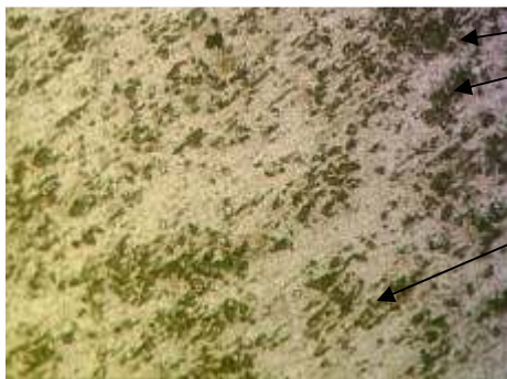
Fig.9-d The microstructure of sample 5 (Top section) 400 X
