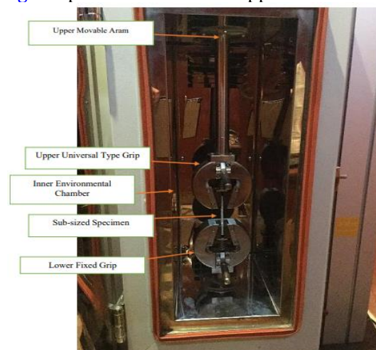
Fig. 2 High-Temperature Tensile Test Specimen Loaded into the Grips with Proper Alignments [15].
