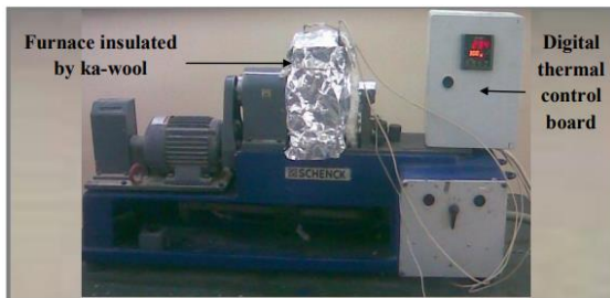
Fig. 4 Furnace Connected to the Fatigue Machine with a Digital Thermal Control Board.
