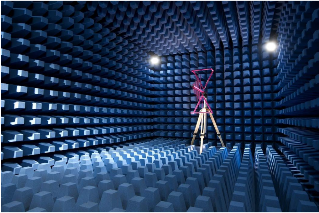
FIG. 5. RF ANECHOIC CHAMBER PREVENTS THE ELECTROMAGNETIC INTERFERENCE BETWEEN TWO OPERATORS [44]
