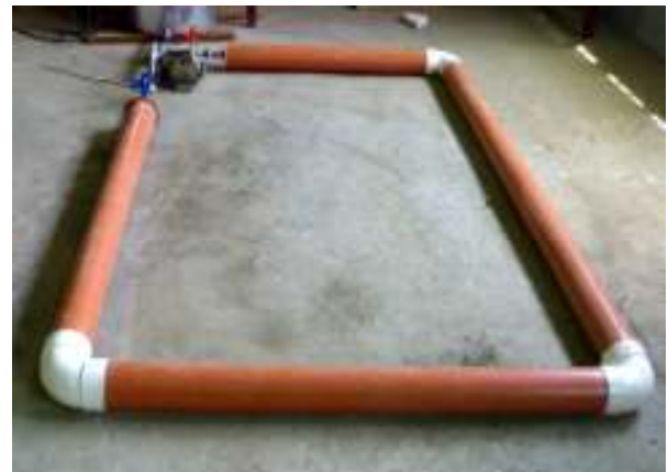
Fig. (6) Photo of pilot loop system of 100 mm diameter PVC pipe
