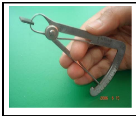
Figure (14) Micrometer metal caliper device used for checking the metal samples.
