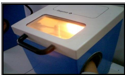
Figure (8): Sandblast machine
