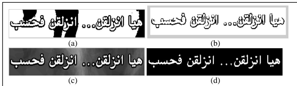
Figure 11. MFI/ Binary level integration. (a) original binary text box image. (b) image I in Eq.9. (c) image AP in Eq.10 (d) image BI in Eq.11 (integrated binary text box image).
