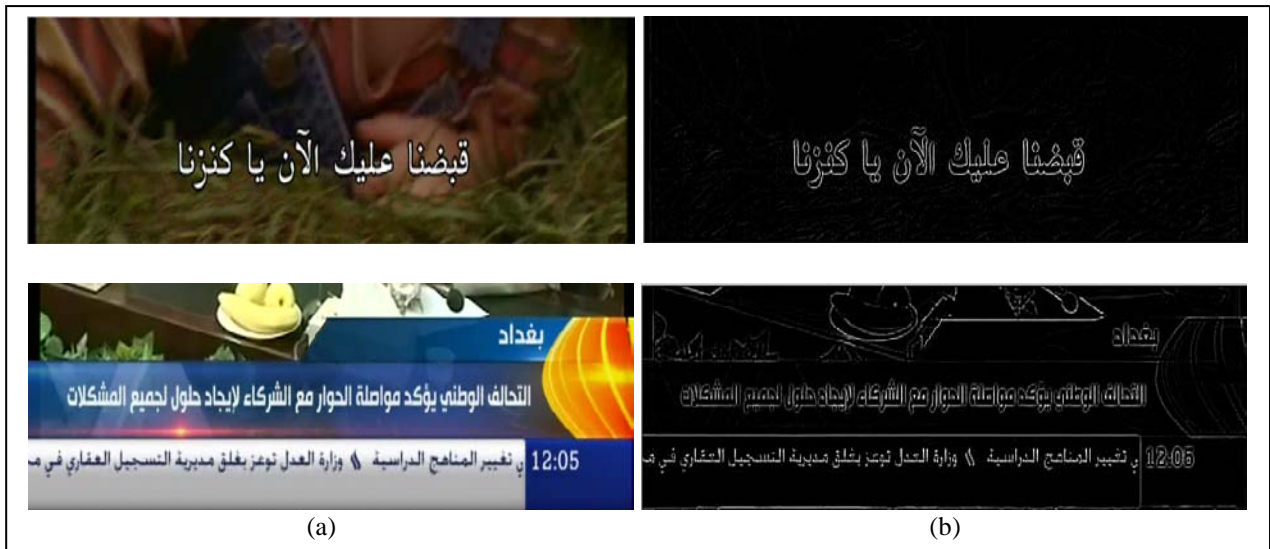
Figure 4. Two examples of using LOG. (a) original true color ROI images, (b) LOG filtered images.
