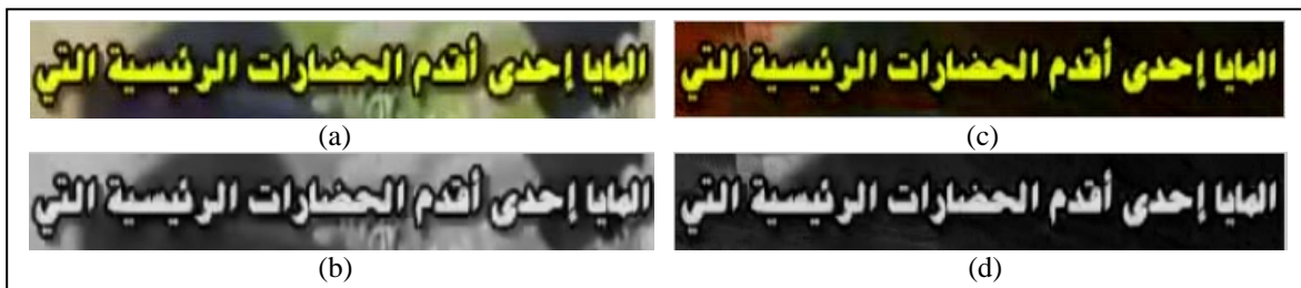
Figure 9. MFI/Gray level integration. (a & b) true color & gray scale text box image respectively. (c & d) text boxes after applying multi frame integration to (a & b) respectively.
