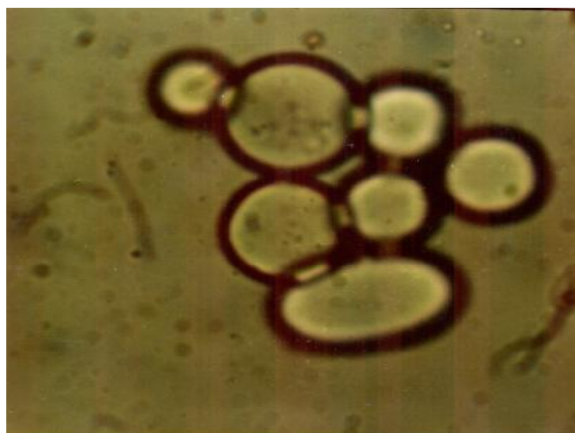
Fig – 3 – Picture of microspheres prepared by coacervation / phase separation method using 30% PLGA
