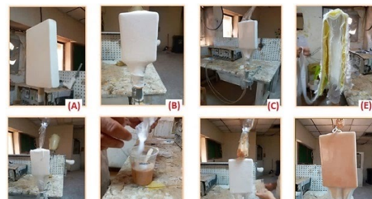
Fig. 3 The Process of Preparing Lamination Specimens for Prosthetic Sockets and Depicts the Various Steps Involved in the Procedure.
