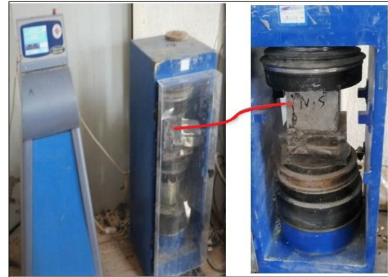
Plate 3 The Compressive Strength Test.
