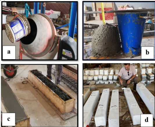
Plate 2 (a) Rotary Mixer, (b) Slump Test, (c) Plywood Molds, (d) Painted Beams.
