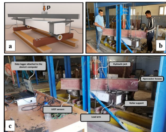
Plate 4 (a) 3D Model of Testing Machine, (b) Loading Frame, (c) Test Machine.
