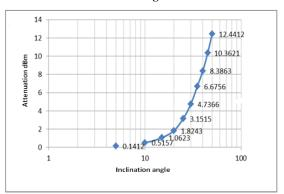
Figure (12): Semi-log chart of Attenuation versus inclination angle between end two faces of fibers at 660nm wavelength.
