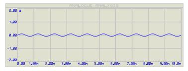
Figure (16): Attenuation in analog sine wave 850nm wavelength & fiber (plastic) where  $v_0$ =0.2v , T=10Sec , v (offset)=0.8v , V (gain)=0.04v and length = 5m.
