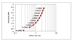
Figure (10): Semi-log chart of Attenuation versus distance between end two faces of fibers at 660nm wavelength
