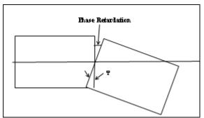
Figure (2): Attenuation introduced by axes rotation or Tilt angle of two spliced fibers
