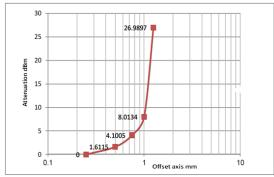
Figure (11): Semi-log chart of Attenuation versus axis offset between end two faces of fibers at 660nm wavelength.
