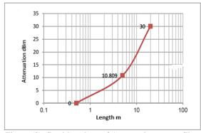
Figure (9): Semi-log chart of Attenuation versus fiber Length at 850nm wavelength
