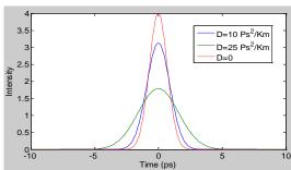
Figure (17): Unchirped Gausian Pulses at Deferient Values of Dspersion along Fiber Optic, nt=512,Tmax=17, z=0.08Km.
