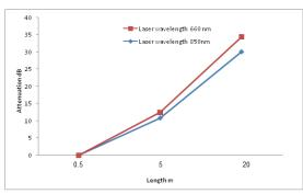
Figure (7): attenuation versus fiber Length at 660nm and 850nm wavelength
