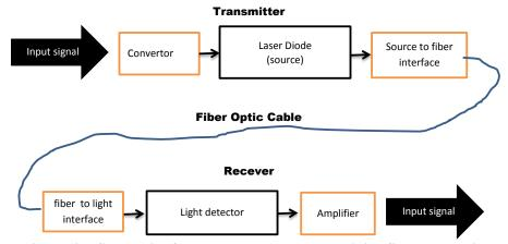
Figure (3): Schematic of laboratory set-up to determining fiber attenuation
