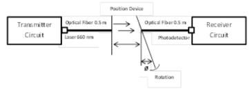
Figure (6): Block diagram for Measurement of attenuation dependence on angle deviation and measurement of numerical aperture
