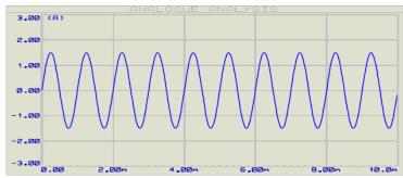
Figure (13): Attenuation in analog sine wave 660nm wavelength & fiber (plastic) where  $v_0$ =3v , T=10Sec , v (offset)=0.8v , V (gain)=0.22v and length = 0.5m.
