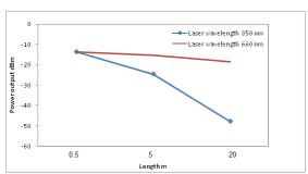
Figure (8): Power output versus fiber Length at 660nm and 850nm wavelength
