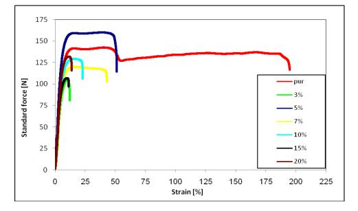
Figure (3) The stress - strain curves and cannabis fiber-LDPE composites.
