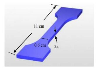
Figure (2) tensile specimen coupon dimensions centimeters.
