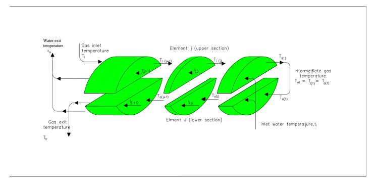
Fig-1- two pass exchanger(heat flow through the differential element)
