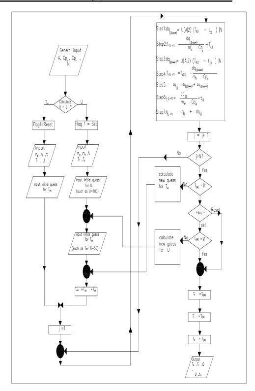
Fig2: Program flowchart for a two-pass heat exchanger
