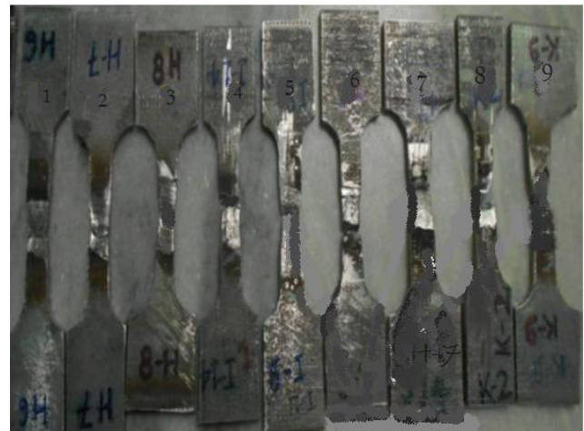
Figure 4: Tensile test specimens.
