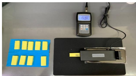
Figure 6: surface roughness tester
