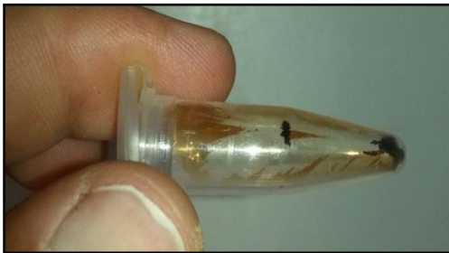
Fig. (3) Appearance of silver nanoparticles after centrifugation
