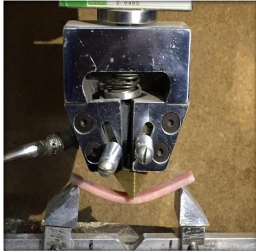
Fig (2): Specimen under stress in instron testing machine
