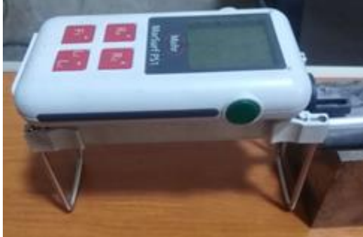
Fig. 3. (Mar Surf PS1) surface roughness measurement device.
