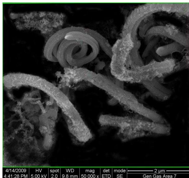
Figure 2: SEM images of the CNFs obtained by \gamma\text{-Fe}_2\text{O}_3 catalyst at 400 °C, and (GHSV) 1600 h -1
