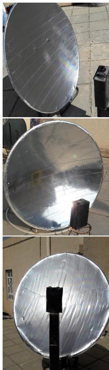
Fig.4 experiments when used a parabolic solar cooker (d=96 cm, 120 cm, and 140 cm) with a 3-liter receiver.
