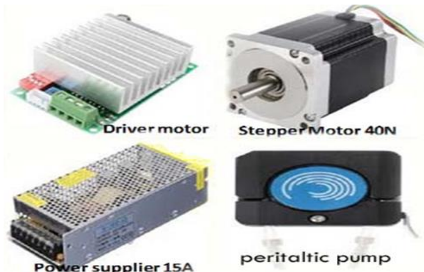
Fig. 2. The comonnents of mini lab made peristaltic pump.
