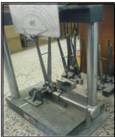
Figure (2): Charpy machine (Impact strength).
