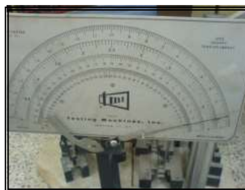
Figure (3): The scale reading gives the Impact energy in (j)
