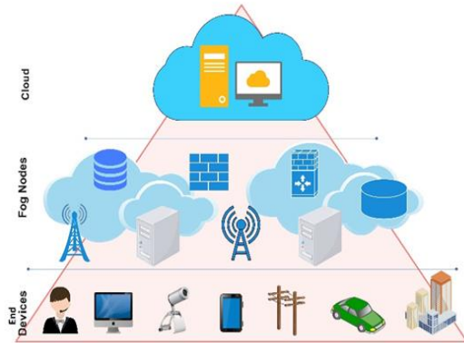
Fig.2 Three-layer architecture (end user/ Fog/cloud).
