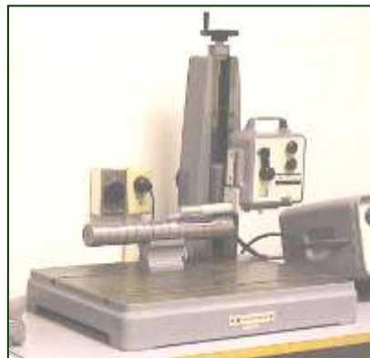
Figure (3): TALYSURF4 machine used to measure surface roughness
