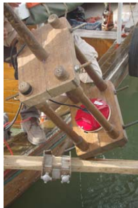
Figure 3. Shows ADCP equipment and its installation during the field work. The equipment was kept at 0.45 m under the surface of water.
