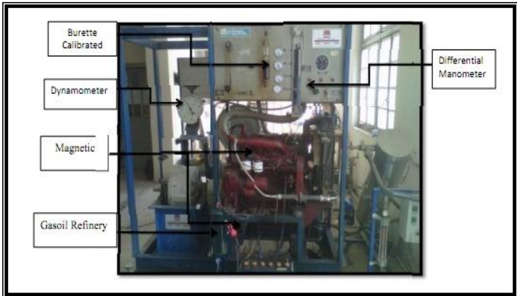
Figure (3): The Experimental Rig of (C.I. engine)
