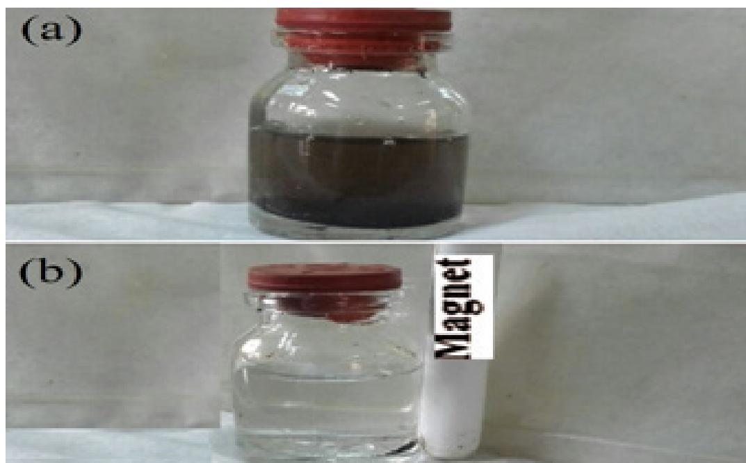
Fig (11): Photographs of the dispersion and separation process of (MRGO-Ar) by magnetic effect: (a) at 5 minute an external magnetic field and (b) after 1 hour an external magnetic field.
