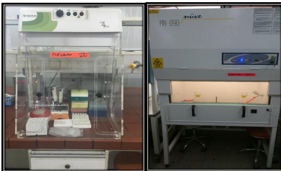
Figure (3) PCR station and biosafety cabinet
