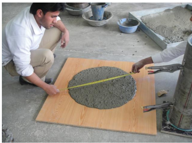
Fig.(2) Stable SCC mixture, no evidence of segregation neither water bled can be seen in the picture (VSI of 0).
