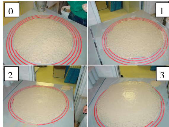
Fig. (1) VSI test ranks the stability of the SCC on a scale of 0-3
