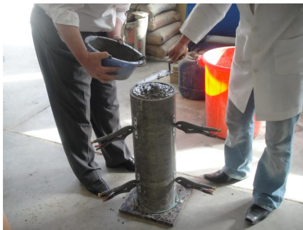
Fig.(4) Column segregation resistance test of SCC
