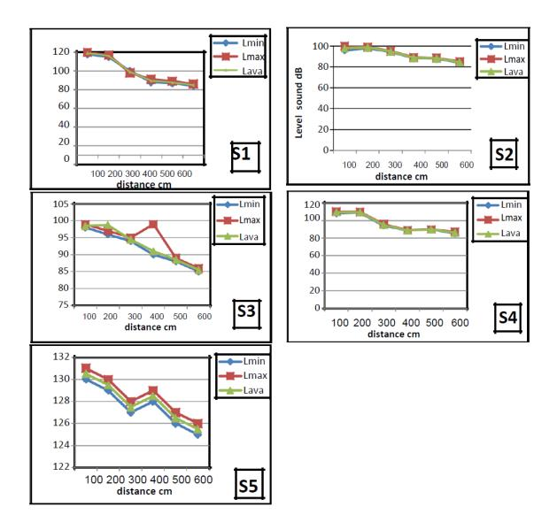
Figures1- 5: Graphs of Sound Level versus Source Distance for the Investigated Sources
